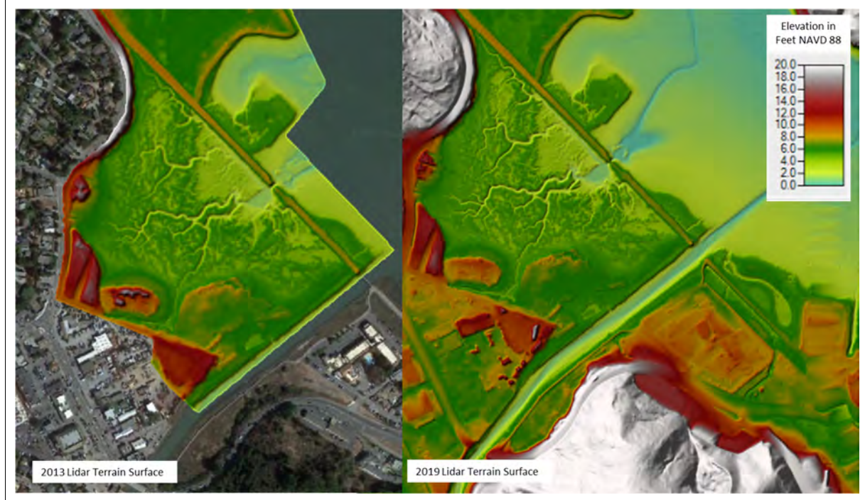
Figure 2-1 LiDAR Terrain Surface Data Coverage of Lower Coyote Creek and Bothin Marsh
